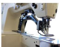
The magnetic clamp ensure high performances and precision during working cycles.
