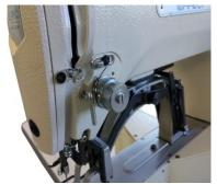
Is possible to store several tension levels depending on used fabric. By selecting the desired one, the electronic thread tensioner will automatically adjust the thread tension.
