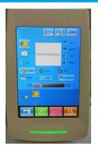
Big sized touch screen panel, suitable to program sewing pattern and data directly on the machine.
